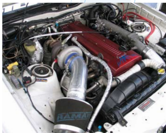
Toyota Soarer with Garrett GT Turbo produces 490bhp to keep the wheels spinning
